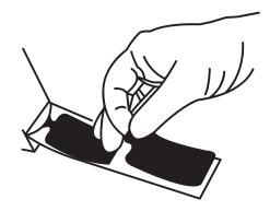
Position the registration mark over center of the injection port.
